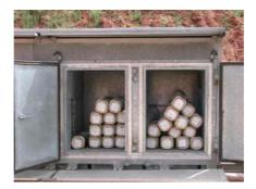
Fig. 1 - Accelerated ageing oven storage
